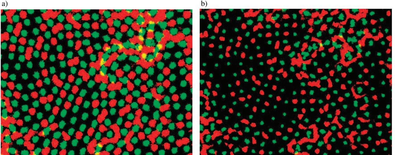
Fig. 2: a) Trajectories of big (in green) and small (in red) particles in the supercooled phase ( $\Gamma = 338$ ) within a box of  $250 \times 180 \mu\text{m}$  and over a duration of  $t = 80000 \text{ s}$ . b) Same as in a) but the trajectories of the particles are calculated relatively to the center of mass of their cage.
